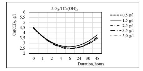
Figure 2. Kinetics of calcium hydroxide sorption-desorption depending on the consumption (concentration) of zeolite
