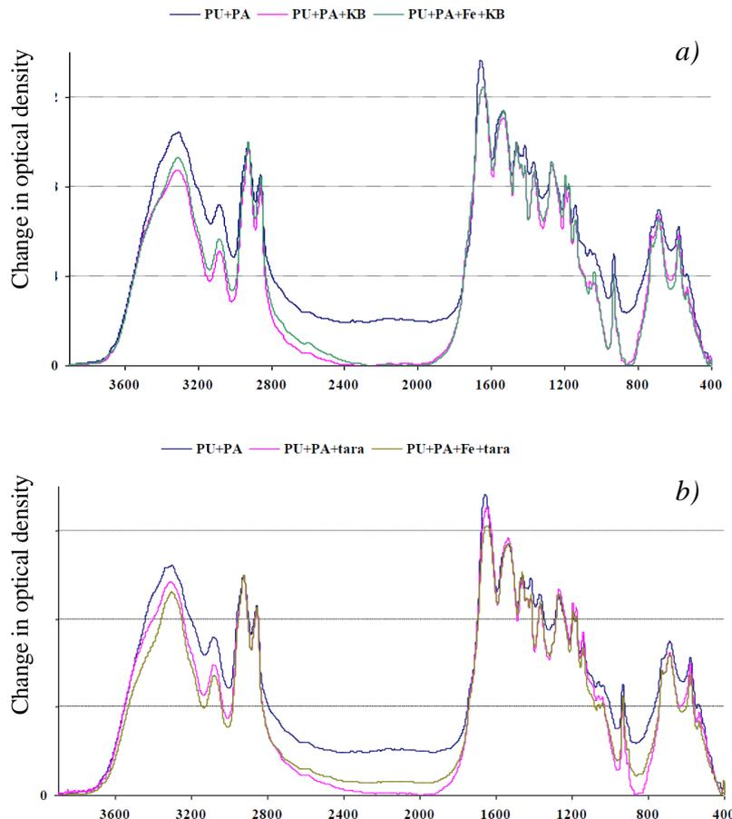
Figure 4. Results of FTIR spectroscopic studies of fibrous sorbent treated by  $\text{Fe}^{3+}$  and polyphenols Quebracho (a) / Tara (b)
