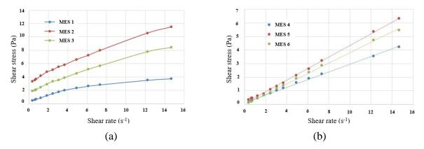
Figure 4. Rheological profiles of shear stress (Pa) as a function of shear rate (s-1) for the tested MES 1 - MES 6 at  $24 \pm 0.5$  °C representing the non-Newtonian flow (a) and Newtonian flow behavior (b)
