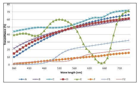
Figure 2. Transmittance spectra of transparent leathers
