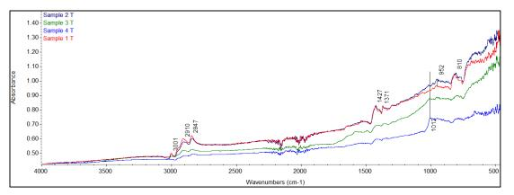
Figure 2. FTIR spectra of vulcanized rubber samples from used tires (coded 1T-4T)
