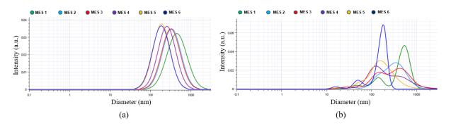
Figure 3. Cumulative profiles of intensity (a.u.) as a function of diameter (nm) analyzed based on Cumulant model - case (a), and profiles of intensity (a.u.) as a function of diameter (nm) analyzed based on SBL model – case (b).
