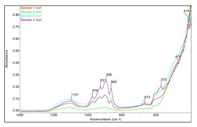
Figure 5. FTIR spectroscopy of ash, coded 1-4 Ash
