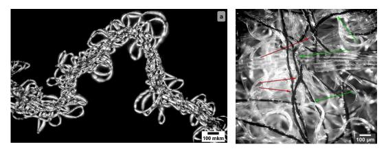
Figure 1. Microphotographs of the fibrous textile wastes: a) high-volume combined loop threads consisting of two components; b) the surface of the non-woven material in reflected light after the thermobonding process
