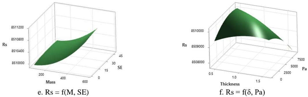
Figure 2. Surface resistance depending on thickness ( $\delta$ ) and mass (a), thickness and SE (b), air permeability (Pa) and SE (c), mass (M) and air permeability (d), mass and SE (e), respective thickness and Pa (f)
