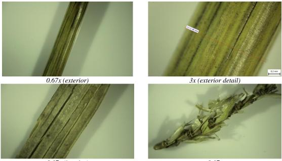
0.67x (*interior*) 0.67x Figure 5. Optical microscopy wheat straw (source 1)
