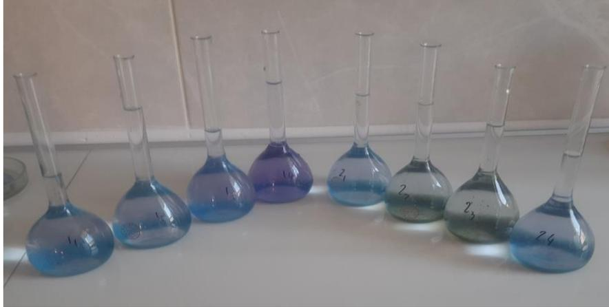
Figure 2. Flasks with analytical solutions prepared for use on the spectrophotometer (first four flasks on the left – after 0.5 h of bating, last four flasks on the right – after 1.0 h of bating)
