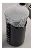
Figure 2. The prepared conductive carbonic paste
