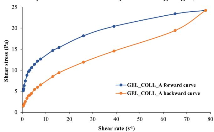
Figure 2. Ascending and descending shear rate versus shear stress curves of perch collagen gel, recorded at 24°C
