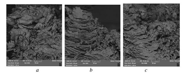
Figure 2. Electron microscopic images of cross-sections of leather samples in the ablation zone: a – Crust leather; b – Flotar leather; c – Nappa leather
