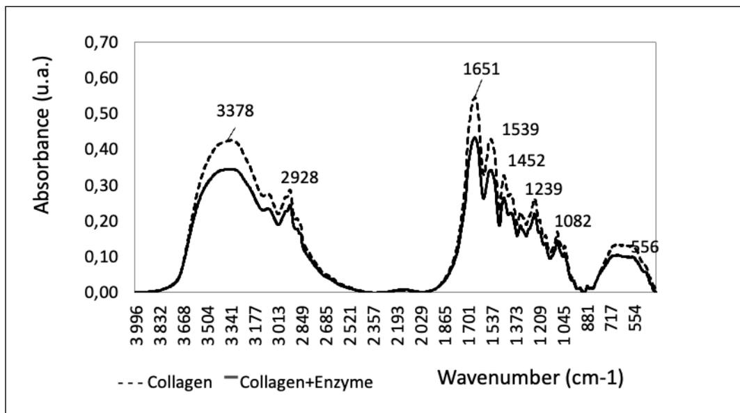
Figure 1. IR spectrograms of collagen preparation before and after treatment with an enzyme preparation
