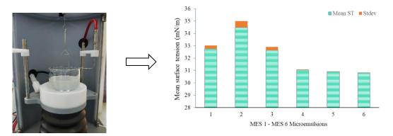
Figure 5. Variation of surface tension for the tested MES 1 - MES 6 at  $24 \pm 0.5^{\circ}$ C, analyzed with Du Noüy ring method
