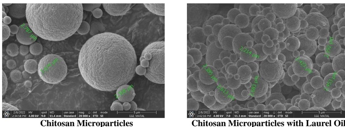
Figure 1. SEM images of microparticles
