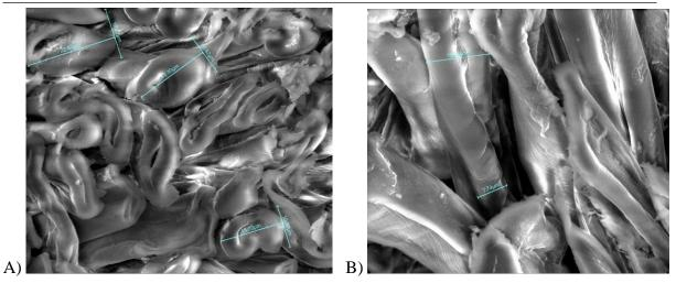
Figure 6. Cotton fibres SEM images: A) transversal section; B) longitudinal
