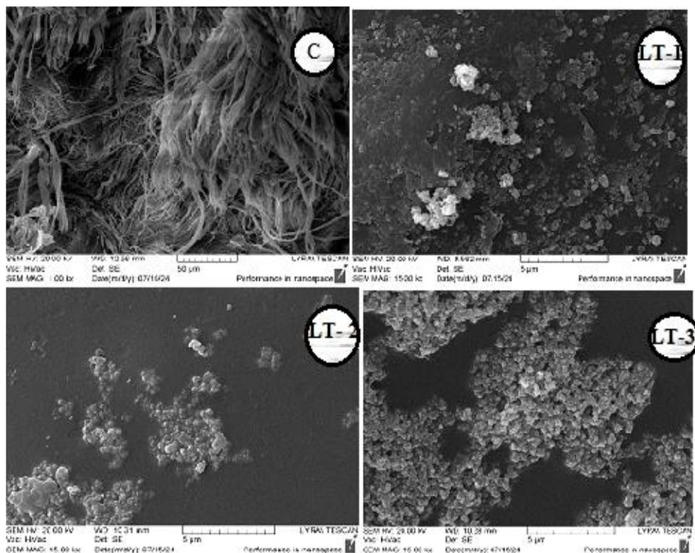
Figure 1. SEM images of the surface of the leather: C – control sample; LT-1, LT-2, LT-3 are modified leather samples
