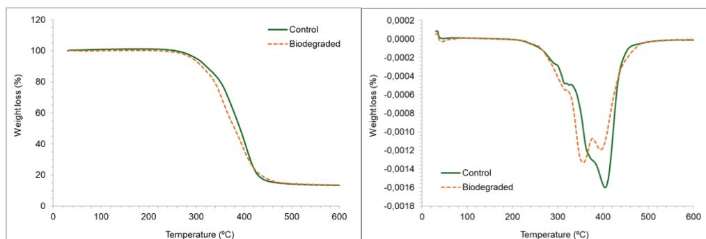
Figure 7. Left. TGA curve comparison of the control and biodegraded samples. Right. DTGA curve comparison of the control and biodegraded samples
