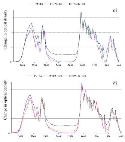
Figure 4. Results of FTIR spectroscopic studies of fibrous sorbent treated by Fe<sup>3+</sup> and polyphenols Quebracho (a) / Tara (b)
