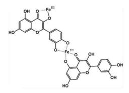
Figure 5. Schematic representation of the coordination interaction of Fe<sup>3+</sup> ions and plant polyphenol molecules according to Walenkcik *et al.*, 2024
