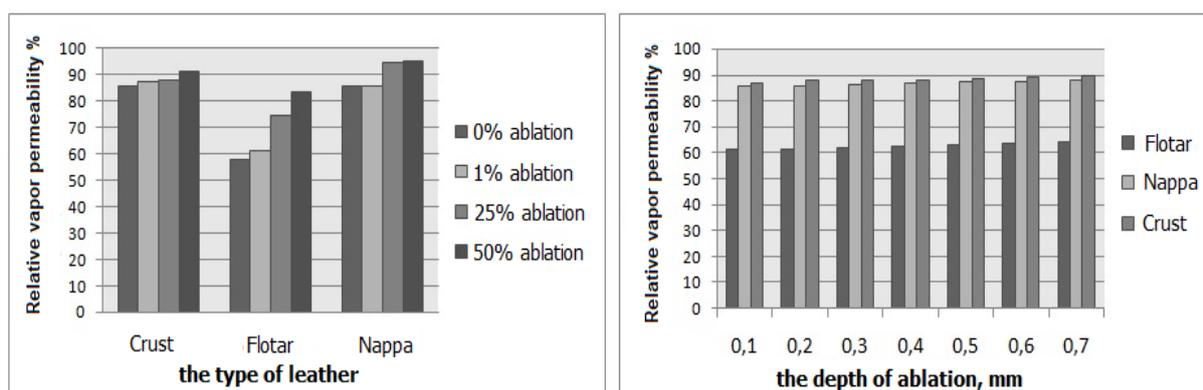
Figure 4. Dependence of vapour permeability on the area and depth of ablation
