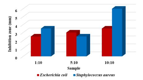
Figure 1. Sizes of the zone of inhibition formed on Petri dishes inoculated with microbial strains and incubated with textile samples treated with ZnO NPs
