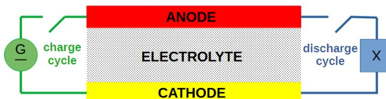
Figure 1. The sketch of electro-chemical storage device
