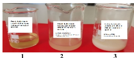
Figure 1. Photographic image of: sample 1 – protein hydrolysates (keratin and collagen) with micro and macro nutrients; sample 2 – protein hydrolysates (keratin and collagen) with micro and macro nutrients + Gemini surfactant (polymethylene-, -bis(N,N-dialkyl-N-deoxy-d-glucitolammoniumiodides); sample 3 – protein hydrolysates (keratin and collagen) with micro and macro nutrients + Bola surfactant (demecarium bromide)
