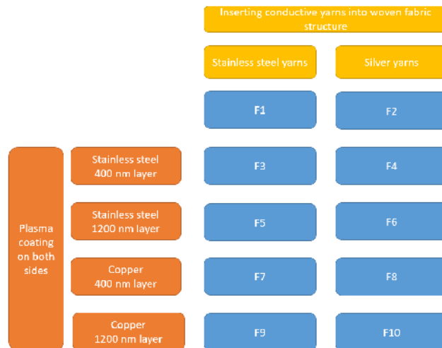
Figure 1. Experimental plan of plasma coating on fabrics
