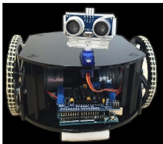
Figure 1. Prototype chassis and component representation of the AGV
